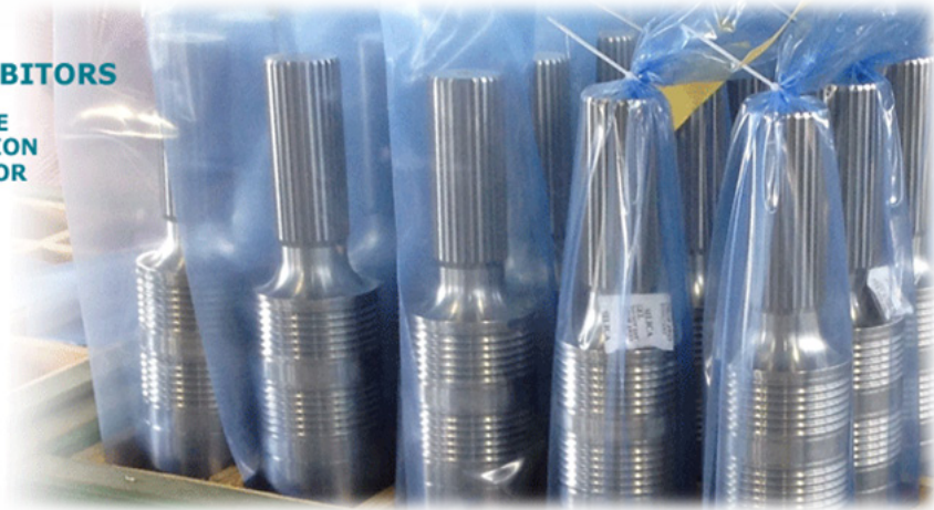
Example of anticorrosion VCI packaging: Vci bags + desiccants
